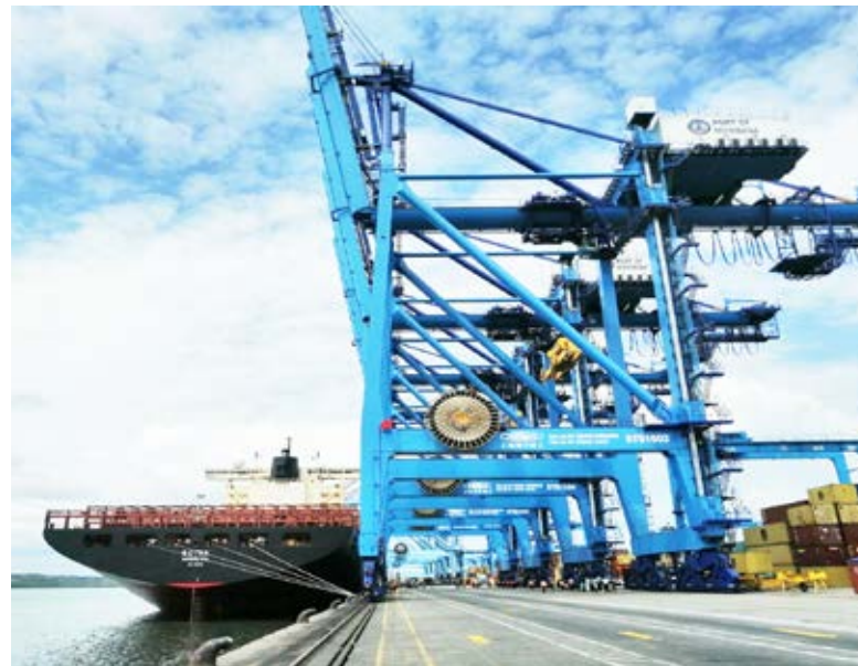
Image of a modern Ship-to-Shore (STS) crane recently acquired by KPA aimed at aiding in unloading of any size of cargo containers at the Port of Lamu
