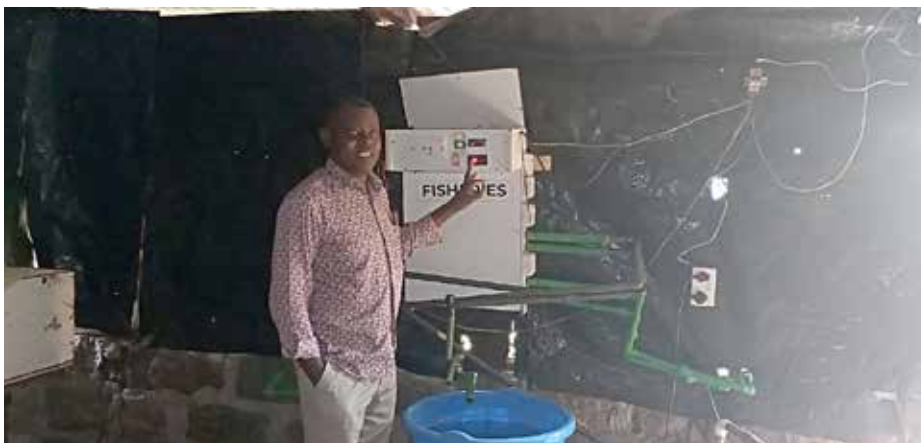
Livingstone Waithaka explains how the Recirculating Aquaculture System works in his hatchery in Ithenguri, Nyeri county. The system maintains the water temperatures in a catfish hatchery at 29°Celsius.
