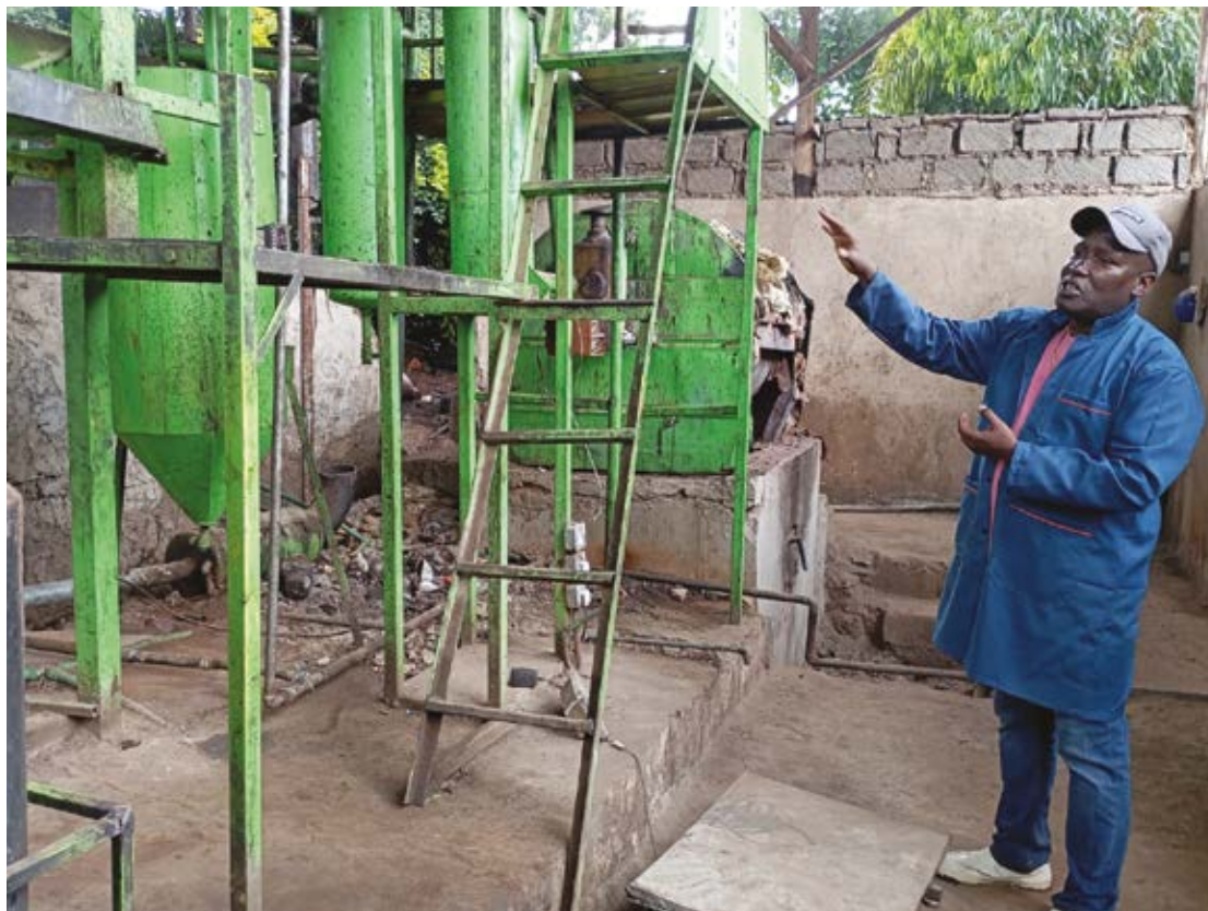
1: Eng. James Muritu at his workshop in Kenol, Murang'a town displays the machinery he uses to convert plastic waste into diesel.
