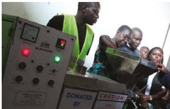
The newly launched milling machine at Muluanda ginnery. The machine with a milling capacity of 80 kg per hour will help add value chain in cotton and improve farmers' profit.
